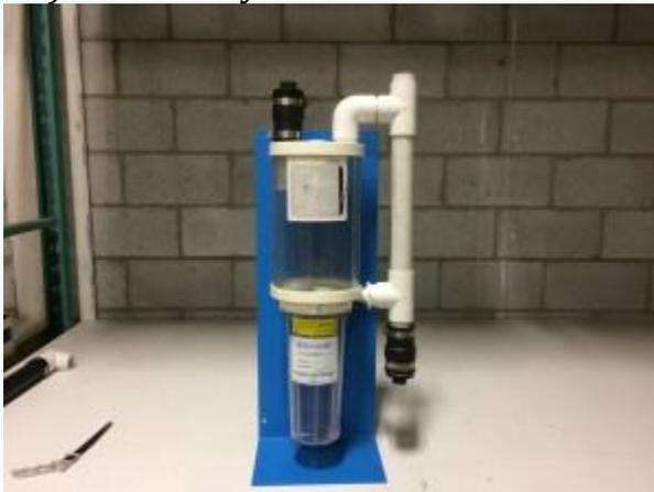
16) If you are upgrading from a filter type amalgam separator; bring out your duct tape to secure the filter to the upper chamber.
