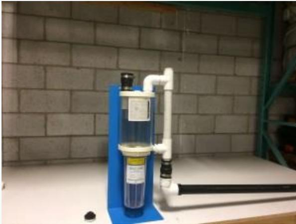
8) Place supplied closeout plug on the inlet of the old amalgam separator.
