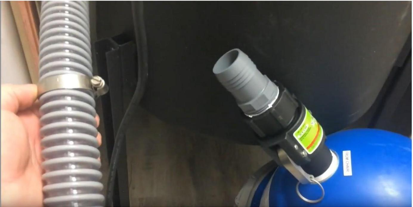
**Step 3** – Use a heat gun and heat the inlet hose, be sure not to overheat.
