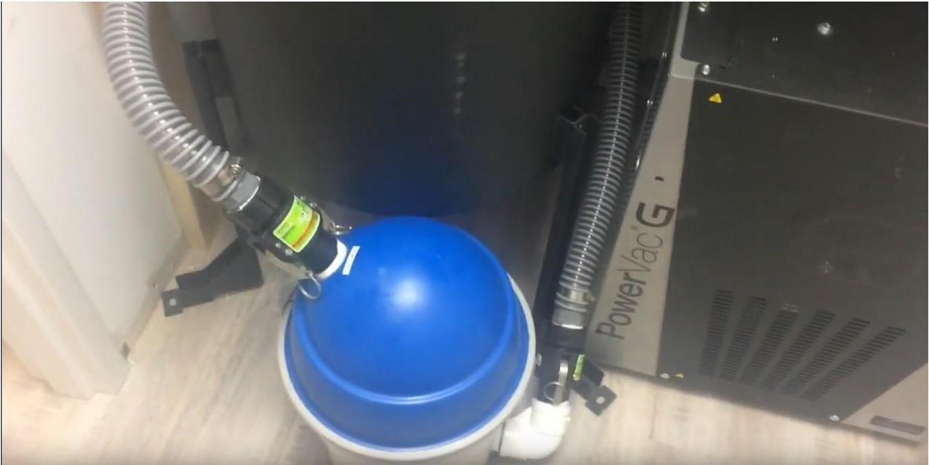
Once you have the outlet fittings attached to the LibertyBOSS, you can measure the length of hose you require to connect the LibertyBOSS outlet to the pump's inlet. With the desired length of hose, you can repeat steps 1-4 from the inlet installation for the barb fittings on the LibertyBOSS' outlet and the pump's inlet.
